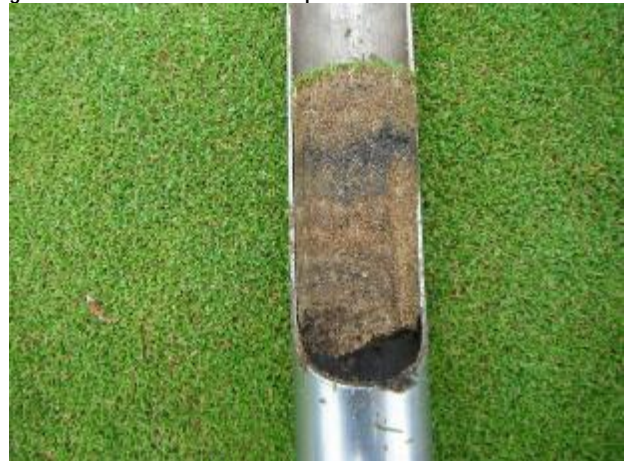
Figure 4: The most organic of all green profiles was the 12 th , which due to higher watering level developed temporary black layer.
